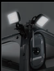
Forward and Left-Facing LED Light (Cab)
